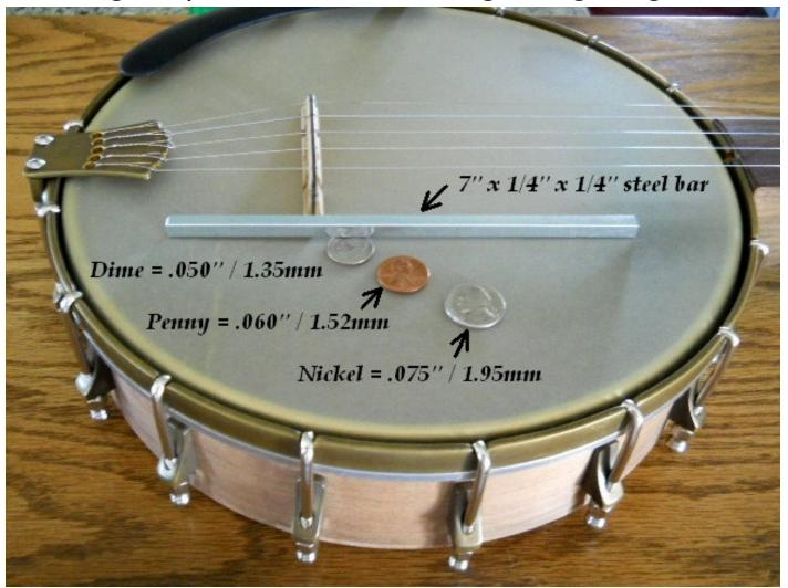
The photo above shows the basic method of checking banjo head tension using a 7" straightedge and standard U.S. coins. The bar is cut from a 12" piece of commonly available hardware store stock; it stands by itself and stores in many case or bag pockets. The photo demonstrates its use with an 11" Renaissance head, 5/8" bridge, no down force from the tailpiece, and using medium steel strings.
